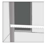
After cutting the panel to length, apply adhesive in a zig zag pattern to the back of the panel or on substrate.
