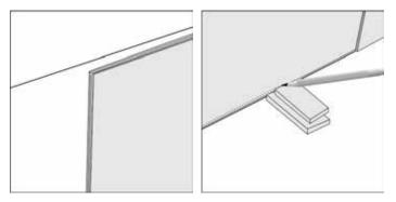
Apply adhesive to the back of the panel. Carefully read and follow the adhesive manufacturer's directions. Apply a 1/4-inch / 6mm bead of adhesive in a zigzag pattern, and a bead around the panel perimeter about 1 inch / 25mm from the edges, or apply by troweling the adhesive onto the substrate, following your adhesive manufacturer's recommendations.
